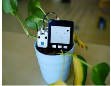
Electrode of the unit is not anti-corrosive, or waterproof, for POC purpose only. Pls do NOT put it in humidity environment for a long while.
