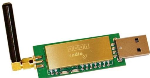
Utilising proprietary LPRS easyRadio technology operating in the 434MHz Industrial Scientific & Medical (ISM) bands the Connect2Pi USB 'dongle' provides a simple 'wireless bridge' between Raspberry Pi (Pi2Pi), a Raspberry Pi and a PC or any other device that supports USB serial communications.
