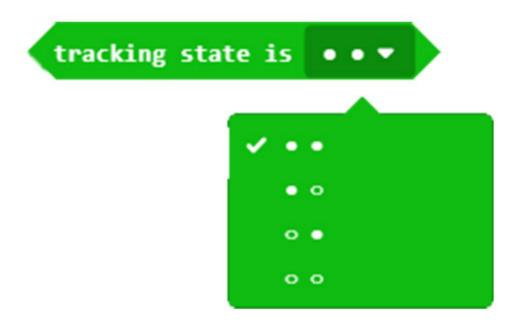
• This brick helps to detect the line-tracking status for the line-tracking modules.
